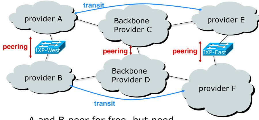
A and B peer for free, but need transit arrangements with C and D to get packets to/from E and F
